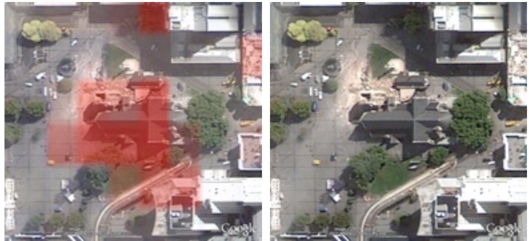
Example of building collapse detected by DPM from Christchurch Earthquake
